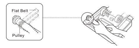
Place the agitator assembly into the grooves in the nozzle head, making sure that the new agitator assembly operate smoothly.
